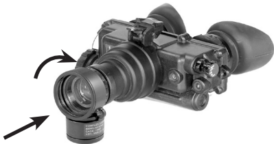
Figure 2-4. Installation of Compass
