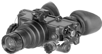
Figure 2-6. Installation of the IR Spot/Flood Lens
