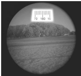
Figure 2-12. View Through Installed Compass
