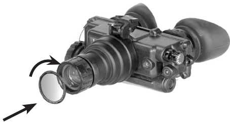
Figure 2-5. Installation of the Light Interference Filter
