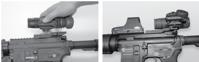
FIGURE 3.3. ATTACHING ATN NVM-14 TO WEAPON MOUNT
