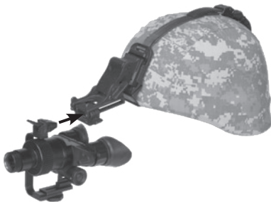
FIGURE 2-15. MOUNT OF NVG-7 WITH ADAPTER TO MIL-SPEC HEAD/HELMET MOUNT INSTALLATION
