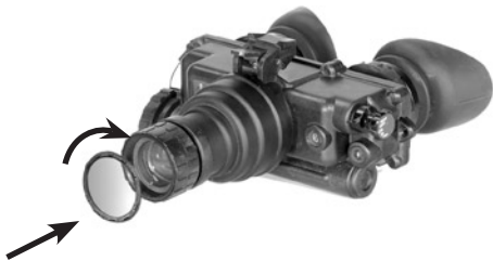
Figure 2-5. Installation of the Light Interference Filter
