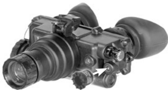
Figure 2-6. Installation of the IR Spot/Flood Lens
