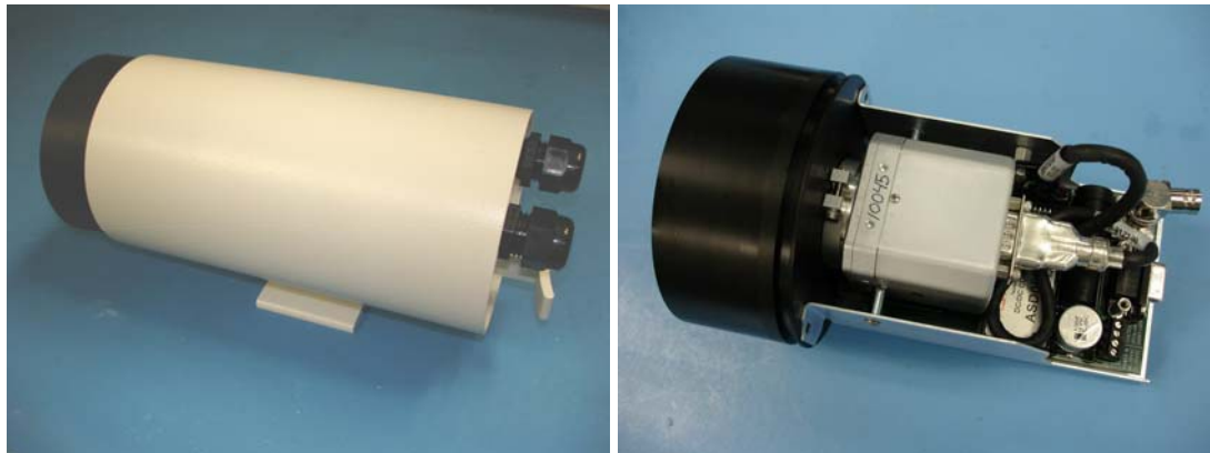
Figure 5: SR-35 Camera with and without the Environmental Enclosure
